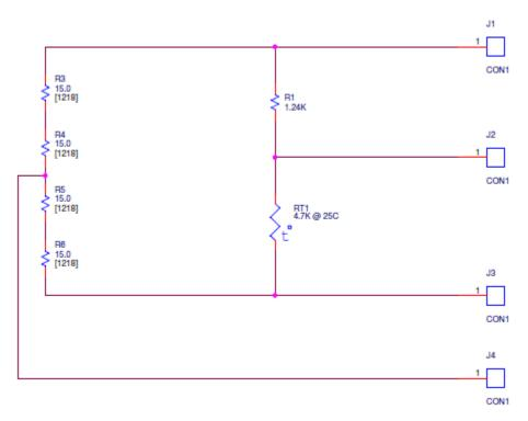
Figure 3.2 Simplified of RF Power Standards Internal Heater
